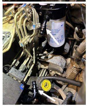
**STEP 12:** Measure and cut the remaining hose to the length needed. Route the fuel hose from the filter block to the VP44 as seen at right.
